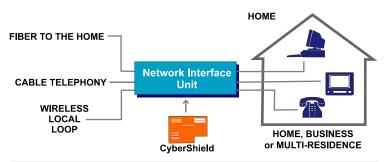
CyberPower CyberShield delivers uninterruptible power to network communications and telephony. Along with providing stable 12VDC or 48VDC power, our units are supplemented with battery backup modules to ensure clean, continuous power, even through power loss. CyberShield products plug directly into network interface units, cable telephony modems, wireless base stations, and fiber to the premise interface modules or integrated access devices.
