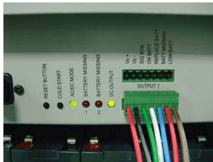
Figure 16: LED's and ONT Alarm Connections
